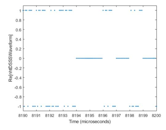
Sample values in DSSS modulation are -1 or 1. The plot shows the real values for a section of the waveform that includes the tail end of the first packet, the 5 microsecond idle period, and the beginning of the second packet for the non-HT format DSSS modulated waveform.
