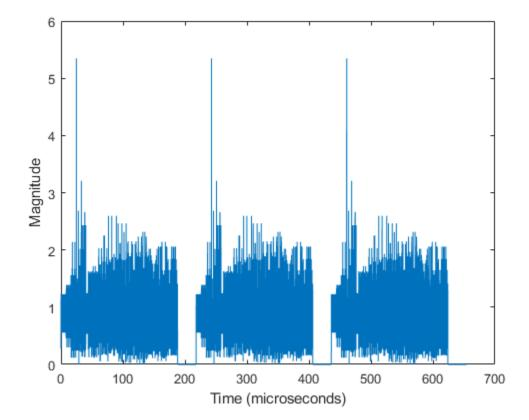
The plot shows three multiuser HE format packets, with each packet separated by 30 microseconds of idle time.
