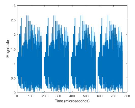
The plot shows four single user HE format packets, with each packet separated by 15 microseconds of idle time.
