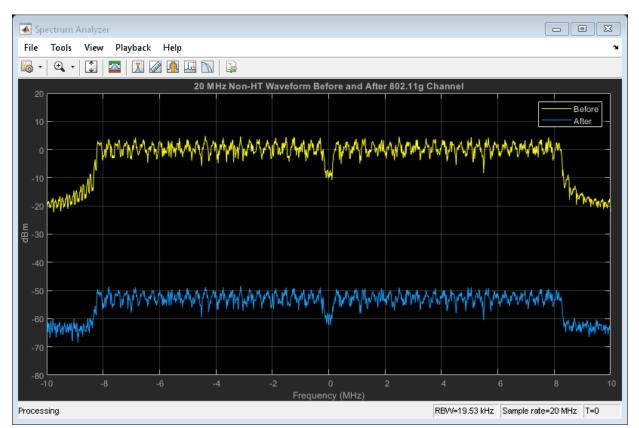
Free-space path loss accounts for the roughly 50 to 60 dB of separation between the waveform before and after it passes through the 802.11g channel. The path loss results from the specified transmitter-to-receiver distance of 3 meters, and from shadowing effects. The signal level variation shows the frequency selectivity of the delay profile across the frequency spectrum.
