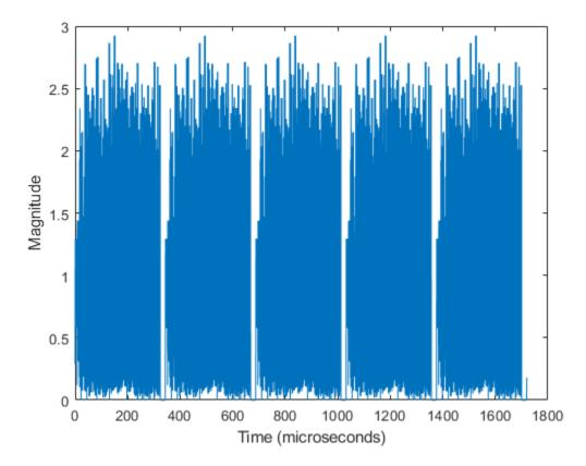
The plot shows five VHT format packets, with each packet separated by 20 microseconds of idle time.
