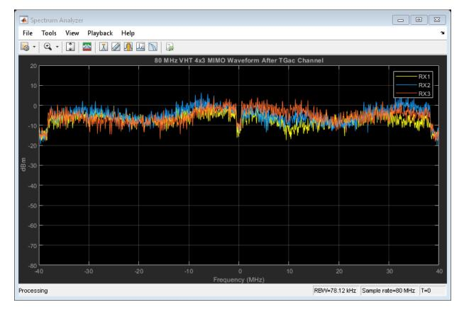
The overlaid signals show the TGac channel variation between the received streams.
