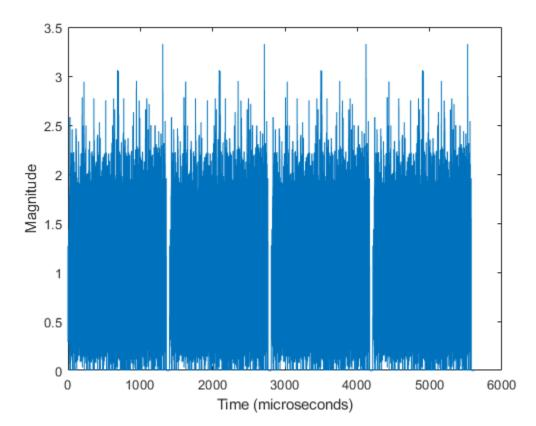
The plot shows four non-HT format OFDM modulated packets, with 45 microseconds of idle time separating each packet.
