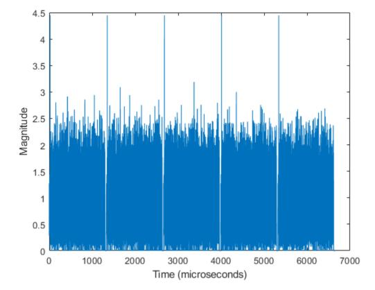
The plot shows five HT format packets, with 30 microseconds of idle time separating each packet.
