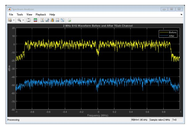
Path loss accounts for the roughly 50 dB of separation between the waveform before and after it passes through the TGah channel. The path loss results from the default transmitter-to-receiver distance of 3 meters, and from shadowing effects. The signal level variation shows the frequency selectivity of the delay profile across the frequency spectrum.
